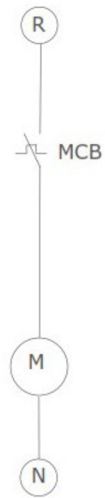
FIGURE 6 - 1 PHASE ELECTRIC MOTOR
